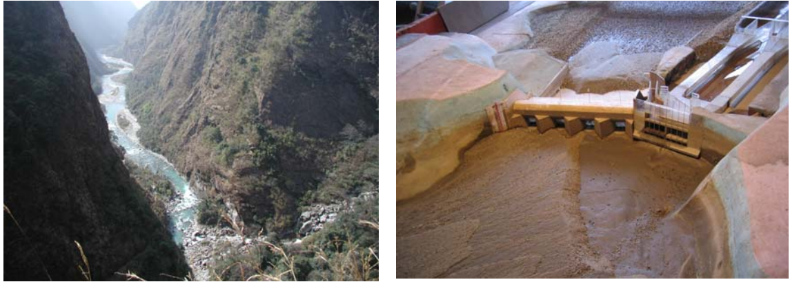
Photo 1: Upper Tama Koshi Hydropower Project: view of river stretch selected for headworks site (left) and 1:60 scale model at Hydro Lab Pvt. Ltd. (Courtesy: Hydro Lab Pvt. Ltd.)
